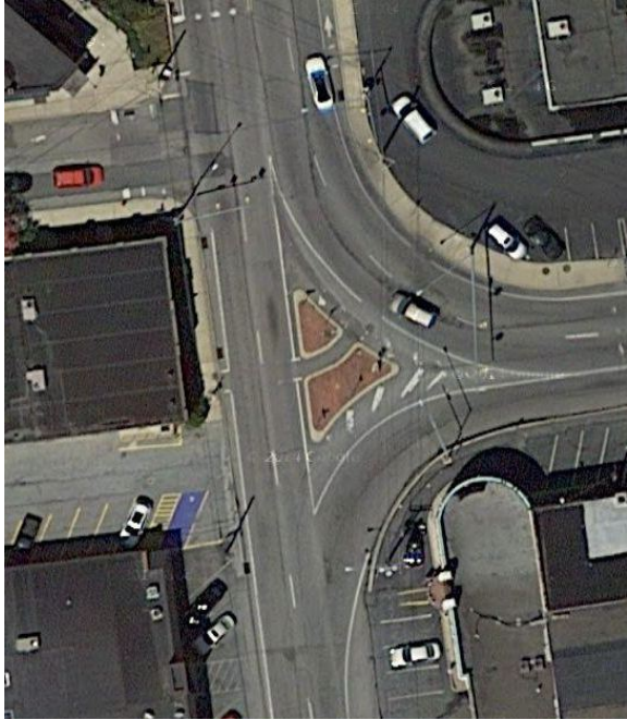
Current: The double-slip-lane configuration at McGovern and Prince encourages both jaywalking and speeding.
