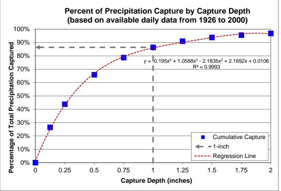
Figure 7.1 - Percent of Precipitation Capture by Capture Depth
